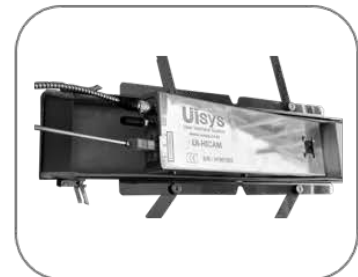
Reflow Inline Camera
